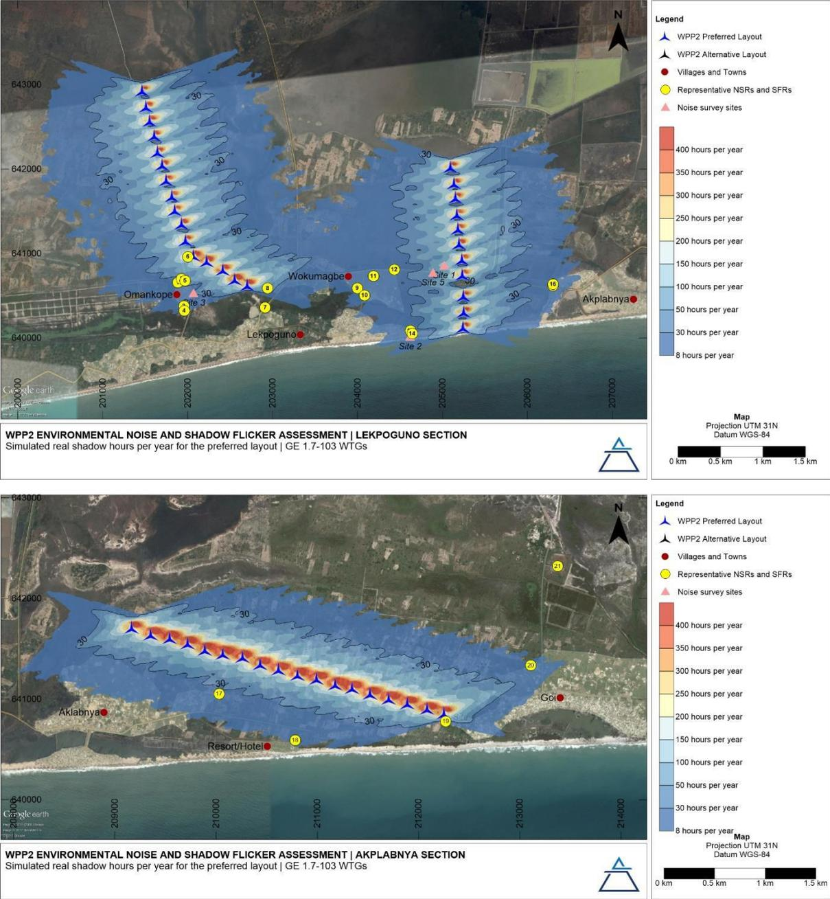
Figure 7-15: Simulated real shadow hours per year for the WPP2 preferred layout
