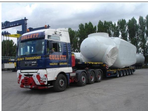
**Figure 3-4: Transportation of a Nacelle**
